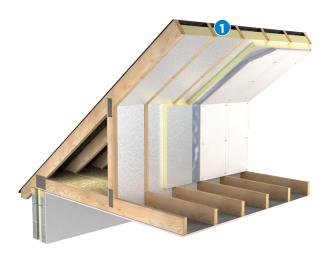
1. In a conventional ventilated roof, a 50mm clear ventilation gap should be maintained between the insulation and the roofing felt. In certain instances, where a breather membrane is used instead of standard roofing felt, the ventilation gap may be dispensed with. Refer to manufacturer's guidelines.
