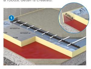
2. Thin-R Underfloor is lightweight and suitable for use with underfloor heating. Thanks to its thickness to performance ratio, it allows for reduced insulation thickness. The boards should be laid with closely butted joints, laid staggered with a break bonded pattern and fitted tightly at edges and around any service penetrations.
